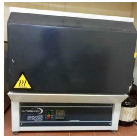
Fig. 4. Photo of the furnace used.
